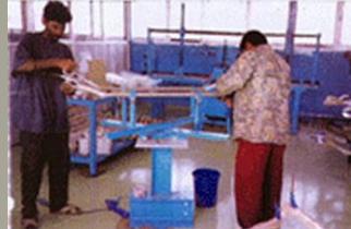
H. T. Coil Insulation taping
