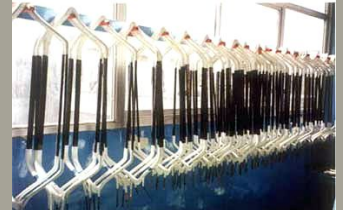
H.T. Coils ready for Mounting
