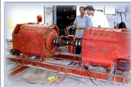
Back to back load testing of DC Machine
